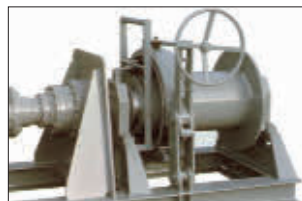
Handbediende bandrem Manual band brake
