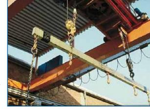
This electrical overhead traveling crane is protected against overload by a PIAB Dynamometer in the hookline anchorage, giving the crane operator the actual load on the hook together with overload. warnings and power shunt.
