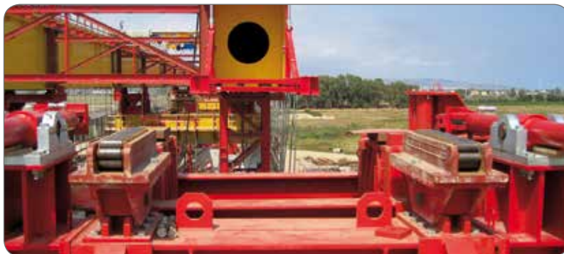
CDE 25/1650 (25 ton, stroke 1650 mm) double-acting cylinder, basculating with plate and pins.
