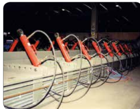
Systems for hot forming large support piles using 22-ton CDE cylinders with Viton gaskets to withstand high temperatures.
