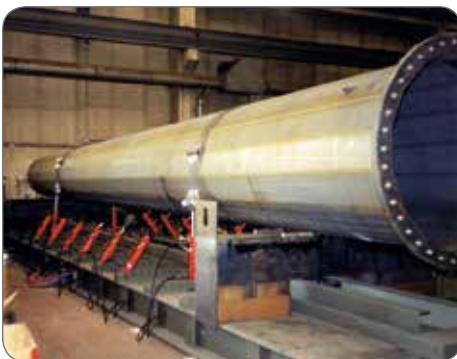
Systems for hot forming large support piles using 22-ton CDE cylinders with Viton gaskets to withstand high temperatures.
