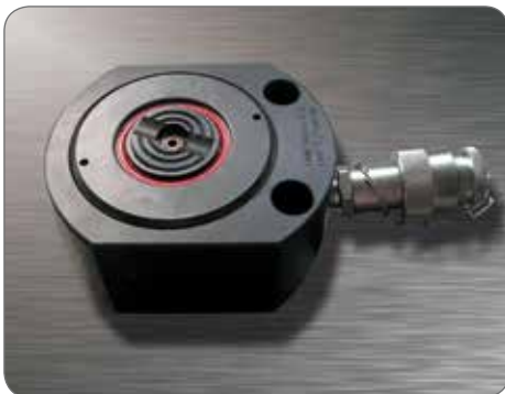
Extra flat cylinder, 50-ton capacity, 16 mm stroke, with built-in self-levelling head.
