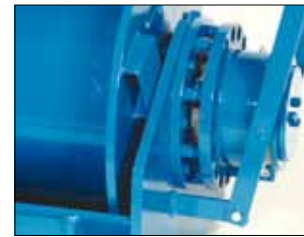
Pennenkoppeling Claw clutch
