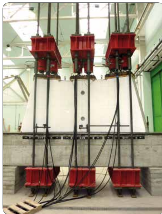
Compression tests in a civil engineering laboratory with 200-ton CRIC cylinders.
