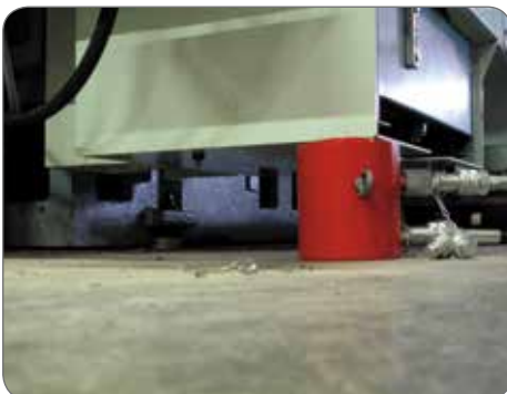
50-ton CRIC for lifting mechanical workshop machinery.
