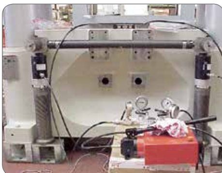
CRMA 50/150 to lift a press section.
