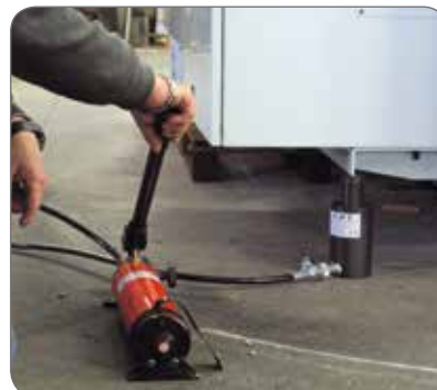
CSE 50/100 for lifting machinery.
