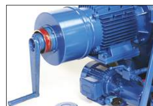
Noodvoorziening (op elektrische motor) Manual emergency crank (on electric motor)
