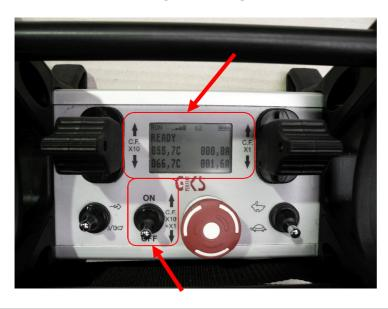
A toggle switch can be used to switch from manual steering to precise straight-ahead driving. This means that only one toggle lever is needed to drive straight forwards or backwards. A corresponding message "SYNC" appears in the display. In addition, the temperature of the two motor control controllers is shown.
