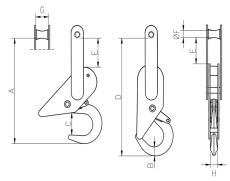
The Automatic Hook Big-C is available in 3 sizes; 2,5 ton, 6,5 ton and 15 ton. It is easy to operate, has rugged design and a high reliability.
